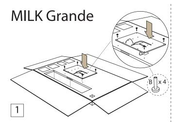
Keep the tabletop in the packaging. The packaging is opened so that the backside of the tabletop is accessible. The top plate is mounted and placed as shown on the illustration. Use the enclosed allen key.
