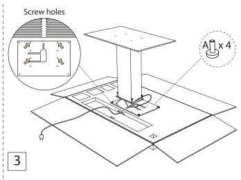
The column with the mounted floor plate is lifted on top of the tabletop and mounted. – see illustration 4.
