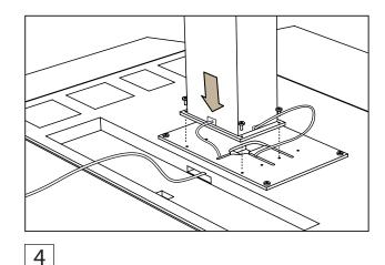
The power cord is let through the cutout in the top plate and into the cable compartment.
