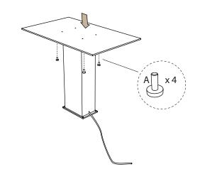
The column is turned with the cable downwards. The floor plate is mounted as shown on the illustration.
